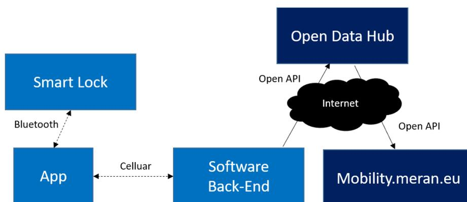
The new bike sharing service is powered by the technologies of the supplier MOQO, a German start-up specialized in IT solutions in the sharing mobility sector, and is characterized by three main components:
